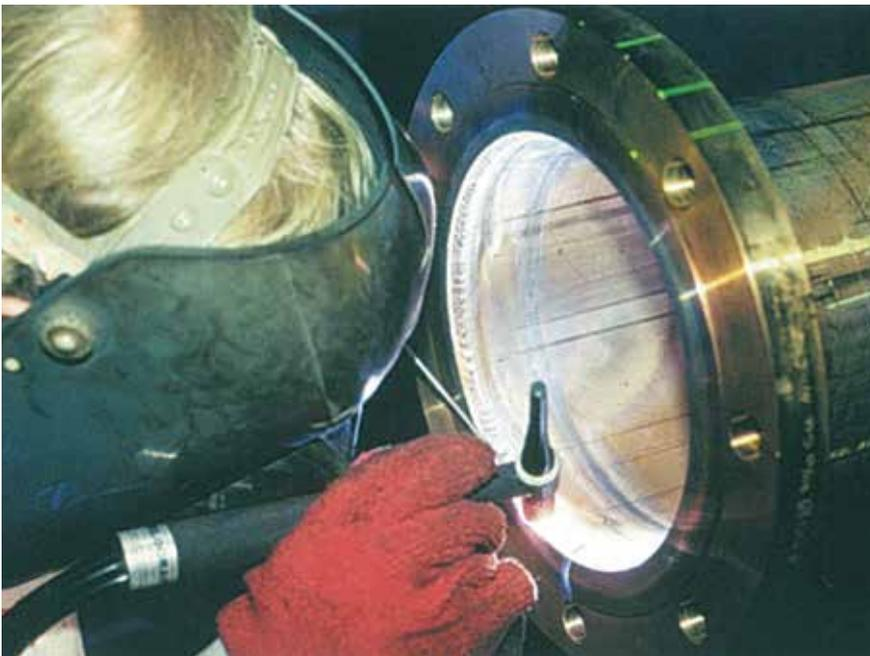
TIG (GTAW) welding a 90-10 copper-nickel assembly
