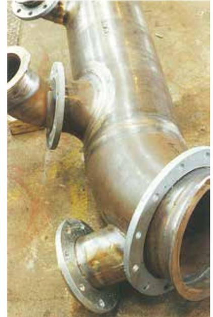
90-10 copper-nickel pipe fabrication for ship seawater system
