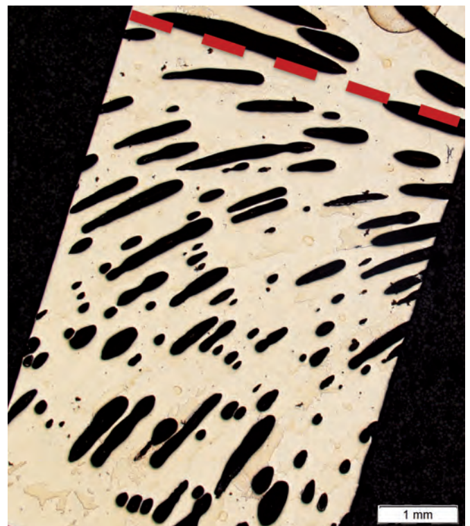
Fig. 17: 17 porosity, cut in casting direction (A.1), center axis marked by dotted red line
