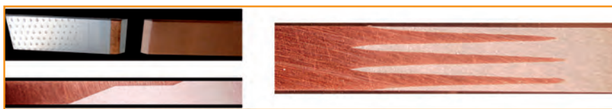
Fig. 5: Initial clad design (left) and resulting Dovetail (right), cross sections
