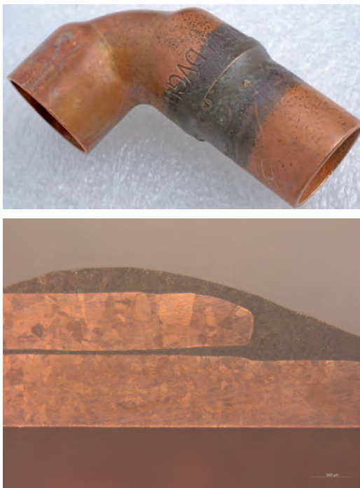
Fig. 5: Brazing of copper tubes with Cu-Ag-P-solder (top: exemplary sample, bottom: corresponding cross-section)
