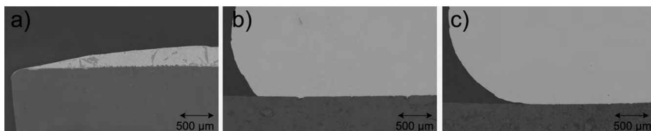
Fig. 1: SEM micrographs of copper on \text{Al}_2\text{O}_3 substrates at 1180 °C for 30 minutes under a) air b) argon c) vacuum
